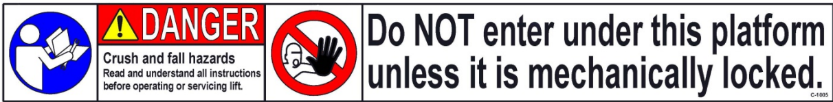
Label #1 placed on all sides of the platform.
