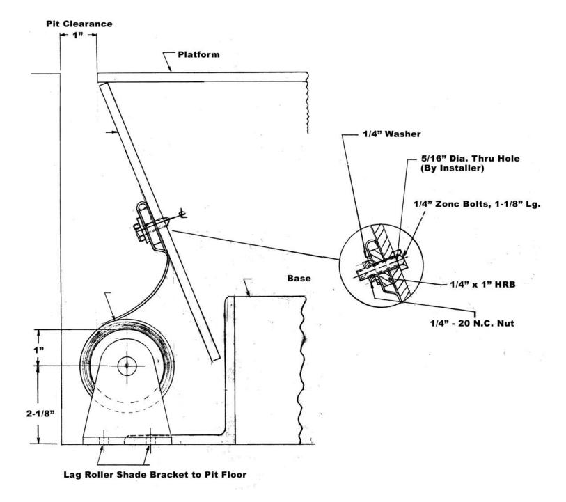
Note: Clamp Hydraulic Line as Required to Clear Shade Rollers.
