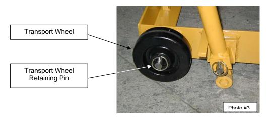
C. Rotate the lever arm assembly in the opposite direction to lower the unit onto the transport wheel. Once the lever arm assembly is resting on the ground, remove the locking pin and repeat the process on the other side of the unit.
