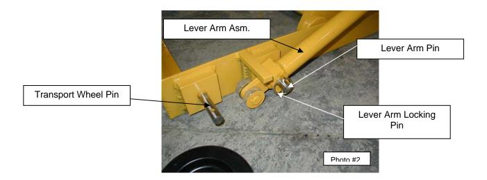
B. Rotate the lever arm assembly upward to lift the unit. Once the unit has been elevated, install the transport wheel on the pin and lock in place with the locking pin as shown in photograph # 3.
