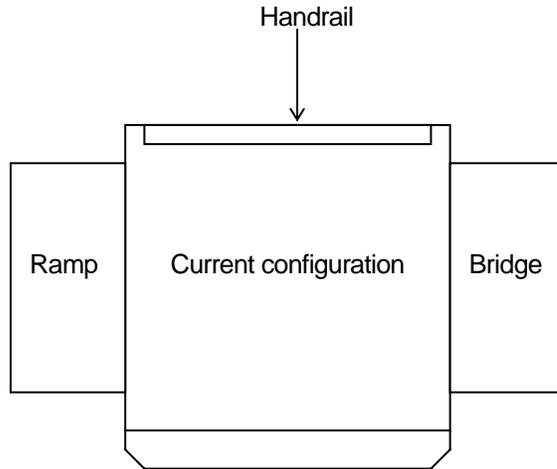
Bridges can be identified by their continuous tube hinges. Ramps are identified by their two pin hinges. All Advance Lifts are designed to accommodate the location of any component configuration. This configuration requires the addition of a pipe stanchion (supplied by Advance) shown in the drawing below, to complete the installation. Please note the mounting detail of pipe stanchion.
