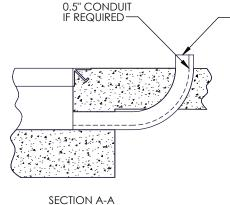
RUN 0.5" CONDUIT & 3" CONDUIT WITH MIN. 14.5" RAD. BEND FROM POWER UNIT LOCATION TO PIT.
