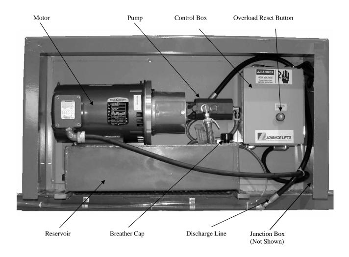
See Page 8-4 for Hydraulic Diagram and Pages 9-3, 9-4 for Electrical Diagram
